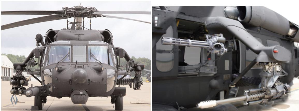
Unitech's LASS weapons pylon are 52 percent lighter when compared to legacy metallic External Fuel System (EFS) pylons, they were designed to replace. LASS wings are easy to install and designed to fit existing UH-60A/L/M Black Hawk variants with standard hardpoints. Unitech looks forward to continuing support of the US government and our allies with LASS solutions for the global fleet of MH-60/UH-60 helicopters.
